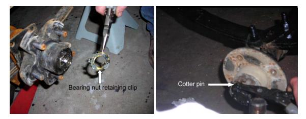
Remove the large bearing nut and flat washer from the axel then remove the hub from the axel.
