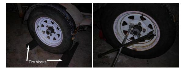
Jack up the side of the trailer where the bearing set is going to be replaced by placing the jack under the axel or under the frame close to the tire. Place jack stand(s) under the frame or axle to ensure that the trailer does not fall suddenly.
