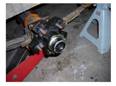
Replace the wheel and tighten all lug nuts. Remove the jack stand and carefully lower the jack. Perform a final tightening on all lug nuts with the wheel on the ground.
