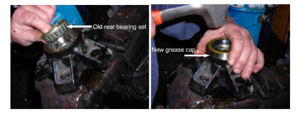
Place the new bearings in the front side of the hub so it sits in the race. Place the flat washer on and tighten the nut until the hub is snug. Spin the hub around a little then loosen the nut about  $1/16^{th}$  of a turn. Make sure that the hub moves freely but that it not "sloppy" (space) between the back of the hub and the axel.
