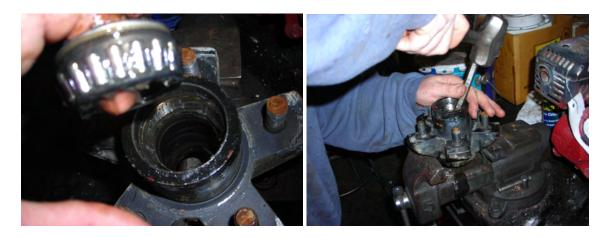
Clean all grease and metal shavings from the inside of the hub. Brake or carburetor cleaning does an excellent job of removing the grease. Also make sure to clean the axel of all grease and metal shavings/parts.
