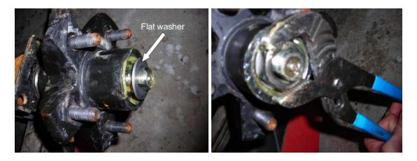
Put on a new retaining clip (or, sometimes cotter pin) and add grease to the bearings until it is full.
