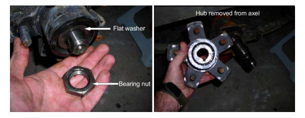
Make sure that you remove ALL of the bearing parts from the axel. The picture below shows part of the bearing casing still on the axel. This commonly happens when bearings go bad.
