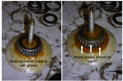
Place the back set of bearings into the hub and tap the grease cover on.
