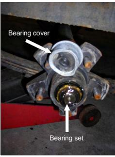
Remove the cotter pin or bearing nut retaining clip. These should be replaced with a new pin or clip during reassembly.
