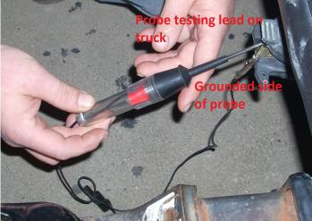
c) If any of the leads shows a failure (light on probe does not go on) a fuse has most likely blown. Refer to the manual in your truck for the location of the fuse(s) and replace it (them).
